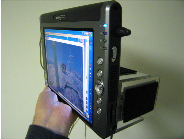
Figure 1. The TabletPC with the sensor rig mounted behind.
